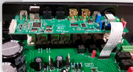
DA200 DAC board on IN100 Signature.
