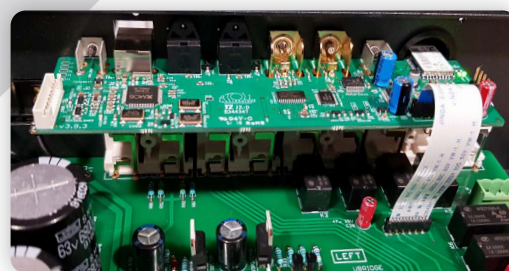
DA200 DAC board in the IN100 Signature
